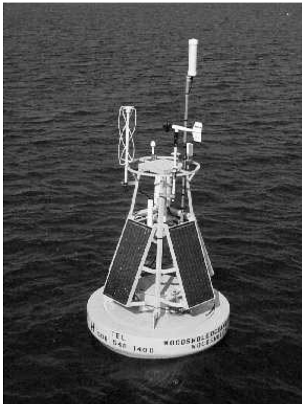
Figure 1. A new steel buoy system (Irish, et al, 1999). The large foam flotation collar is seen as the basic buoy hull. Above the solar panels the tower holds meteorological sensors, the radar reflector, the guard light and an ARGOS locator beacon antenna. The satellite transmitting and receiving antennas are mounted highest on the tower. A GPS receiving antenna for position is also included.
