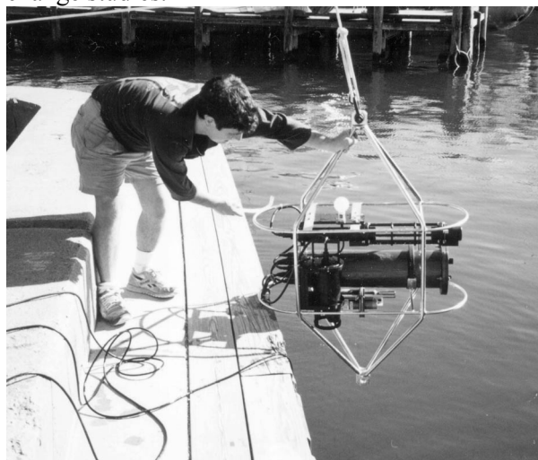
Figure 4. Paul Fucile with a bio-optical package in its mooring frame. The "light bulb" on top is a scalar PAR sensor, the horizontal sensor below the transmissometer, the large horizontal tube in the middle the data system and battery case, the chlorophyll-a fluorometer is on the left bottom, and the Sea Bird temperature and conductivity sensors can be seen lowest in the frame.
