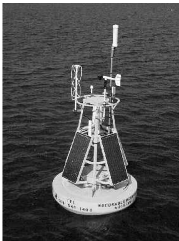
Fig. 1. The new buoy system undergoing full system tests off the WHOI dock. The large foam flotation collar is seen as the basic buoy hull. The tower holds the four large solar panels. Above the solar panels the tower holds the radar reflector, the guard light and an ARGOS locator beacon antenna. On top of the tower the satellite receiving antenna (highest on right) and transmitting antenna (spirals on left) are mounted as far apart as possible.
